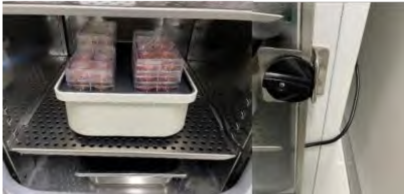
Figure 2. Orbital shaker culture of cardiac organoids at 37°C with 5% CO 2 .
